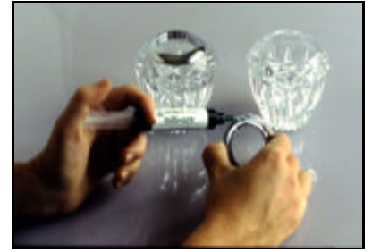
Stainless Steel Trim Bonded to Crystal with DYMAX Light Weld® 619
